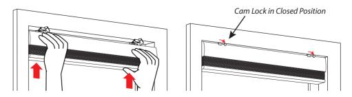
8 Be sure the blind is secured into each bracket before operating the blind.
