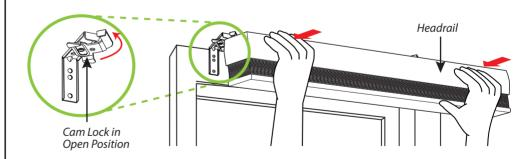
7 Once the blind is in position, push the cam lock toward the headrail to lock the bracket into the blind.
