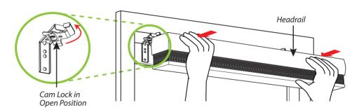
7 Ensure the blind is centered on the window and then rotate the headrail backward toward the window until a 'click' is heard. This means that the headrail is engaged into the brackets.
